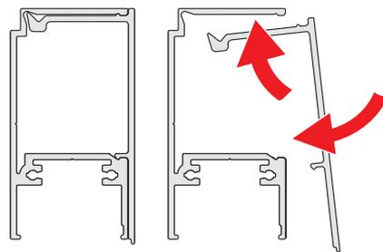
The fixing and internal control are covered by the elegant profile cover.
