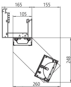
Installation without glazing element possible with Sottezza II
