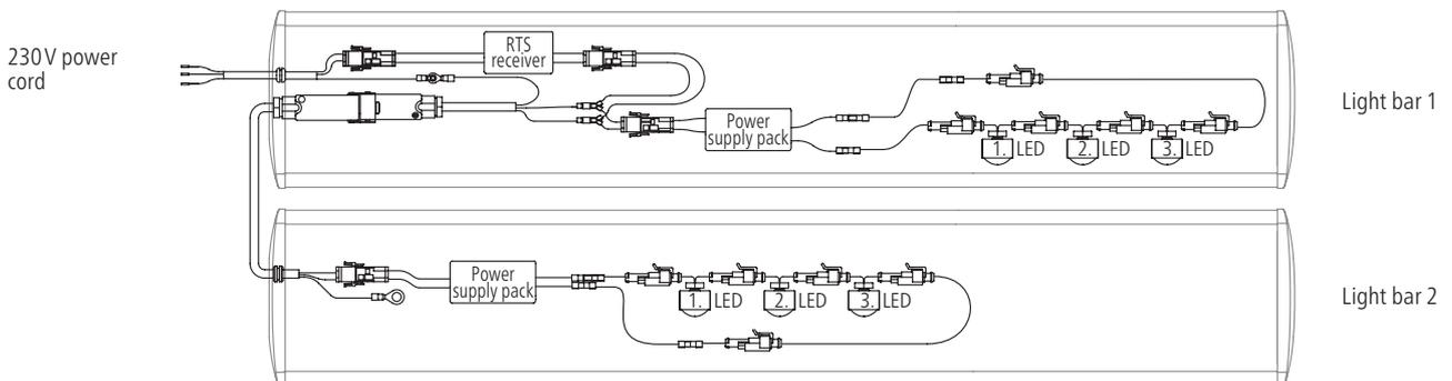
Schematic diagram of light bars for a coupling. Light bars can be designed both individually and with other couplings.
