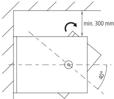
When mounted on a wall, the Tempura Quadra can be swivelled 40°.
