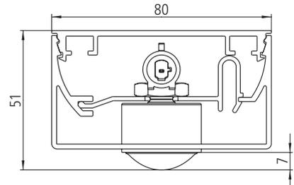
**LED Design 3Spot round/square: position of the LED spotlights and cable output**
