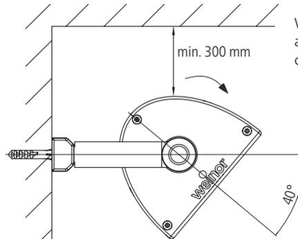
When mounted on a wall, the Tempura can be swivelled 40°.
