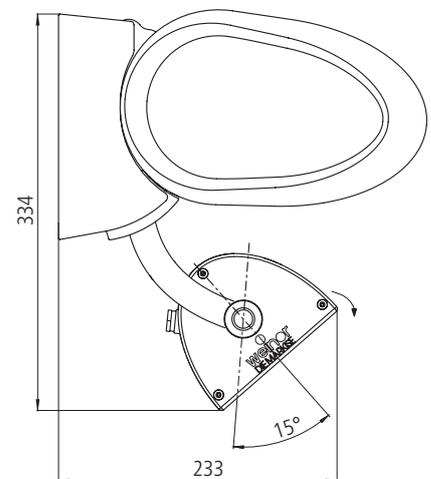
When attached to an Opal Design II, the Tempura Quadra can be swivelled 15°.
